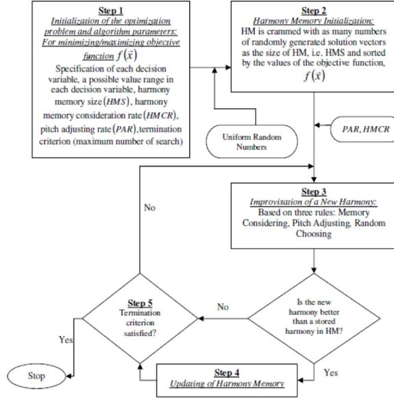
Figure 2. Flow-chart of the classical HS algorithm
