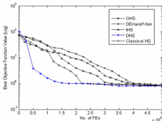
Figure 6. Progress to the optimum solution for spread spectrum radar poly-phase code problem ( $n = 20$ ).
